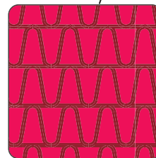
Patented HoneyCombe® wheel design provides a vast surface area for desiccant
